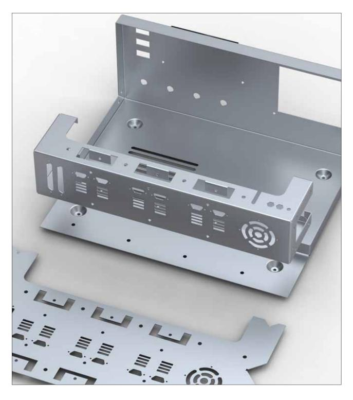
Radan3D is a high performance and versatile 3D modelling package designed to make sheet metal design and engineering assembly modelling simple.
